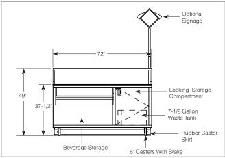
All fixtures and equipment to be connected to a single load center. Cart to have one (1) 8' power cable with a NEMA 5-15P plug.
