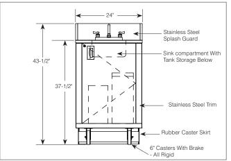
All fixtures and equipment to be connected to a single load center. Cart to have one (1) 8' power cable with a NEMA 5-20P plug.
