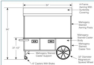
All fixtures and equipment to be connected to a single load center. Cart to have one (1) 8' power cable with a NEMA 14-30P plug.
