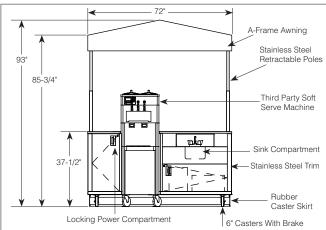
All fixtures and equipment to be connected to a single panel for one point connection load center. Cart to have one (1) 8' power cable with a NEMA 14-50P plug.
