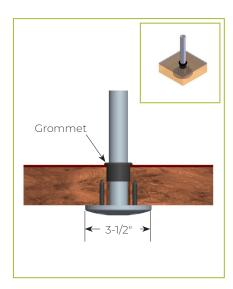
Verify Counter Thickness or Under-Counter Installation Depth in Inches
