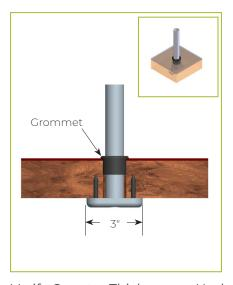
For Millwork Counter MWU4: Compression Installation (not recommended for solid surfaces)
