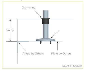
For Stainless Steel Counter (requires under-counter reinforcement and access)
